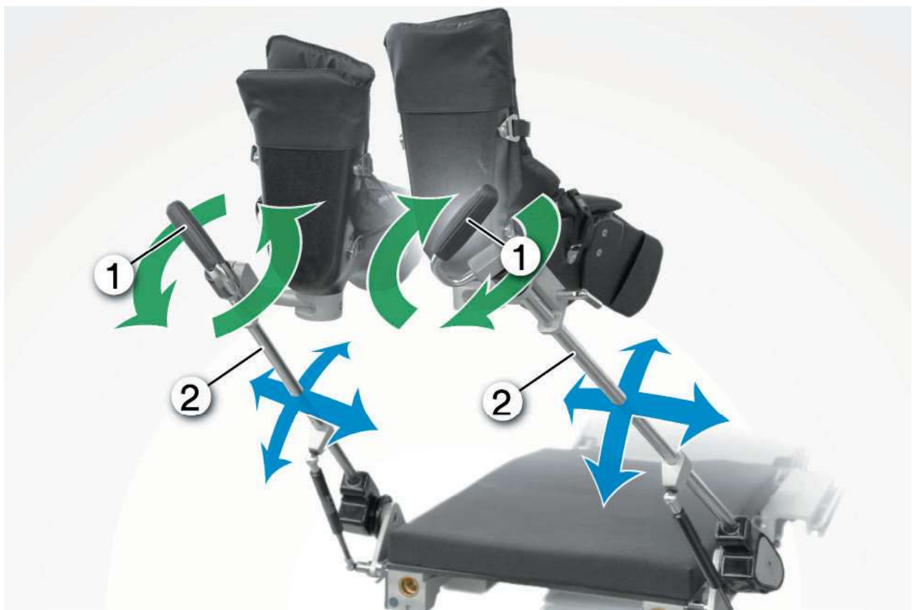
Fig. 10 Turn release handle (top arrows), adjust slide tubes (bottom arrows) 1) Release handle 2) Slide tube
